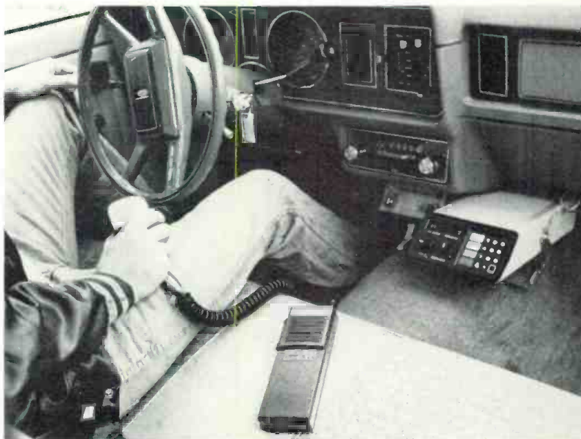
In ENG vehicle used by KLAK/KPPL, 450 MHz radio for link to studio is in space to right of operator. Hand-held transceiver, lying on seat, can use car system as relay to get live material into the studio
