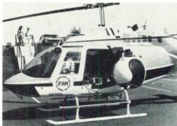
Another approach to getting close-up pictures from helicopter-borne systems is being promoted by Microwave Associates. The IsteC bubble mounted on the helicopter contains a remotely controlled camera with powerful optics. The bubble is stabilized by a tri-axis gyro. FAA STC certification for the unit is pending, but demonstrations have shown pictures taken from an altitude of 1000 feet that appear to have been shot with a normal lens from a vantage point only 50-100 feet away. The Gyro system will sell for about $90,000 to $120,000
